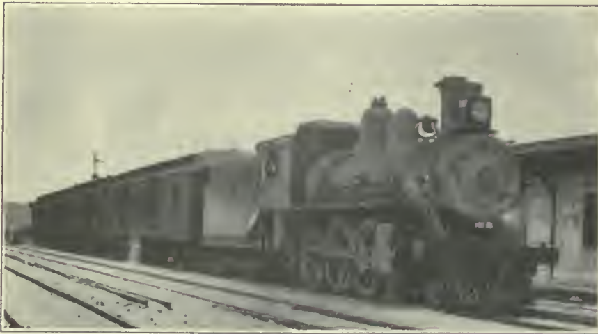
FIG. 372. SUBURBAN PASSENGER TRAINS. Suburban Train of the Pittsburgh, Fort Wayne & Chicago Railway at Englewood Station. This train consists of a ten-wheel locomotive and three coaches.
